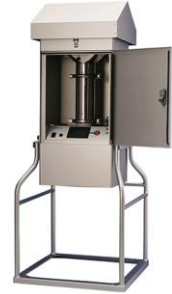
▲ High Volume Air Sampler
