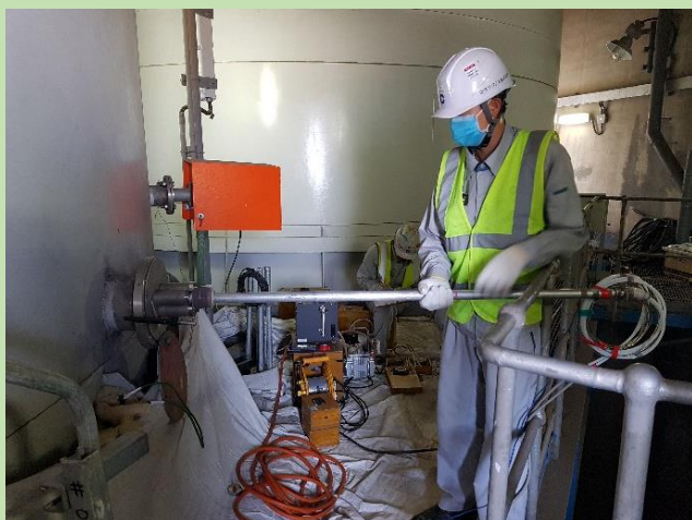
▲ Monitoring of exhaust gas temperature, pressure
